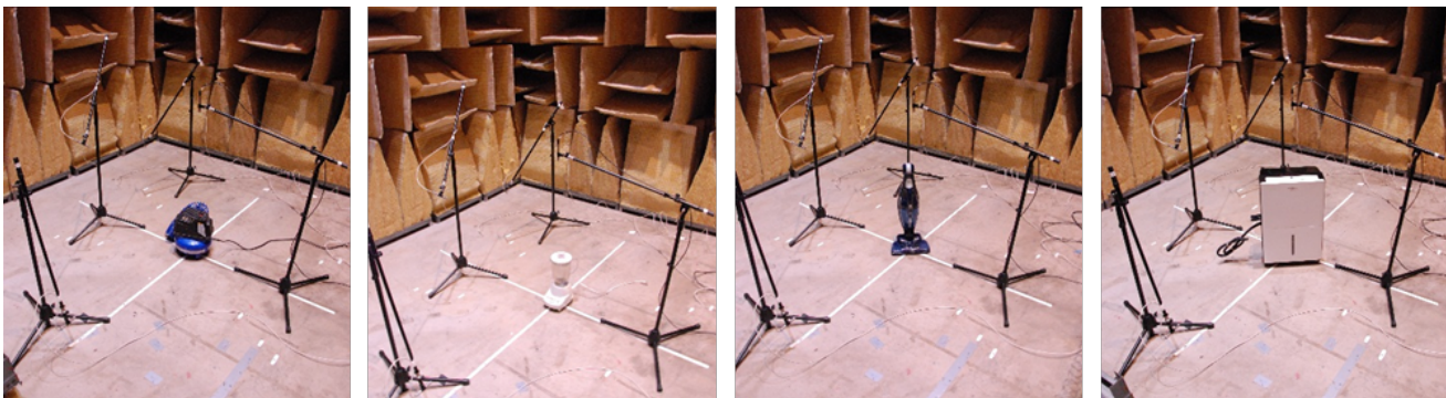
Figure 3. Common household sound sources from left-to-right: 100 psi air compressor, blender/mixer, cordless boom/vacuum, and dehumidifier. The sources are shown in the ARL/Penn State hemi-anechoic chamber with four PCB 378B02 microphones.
